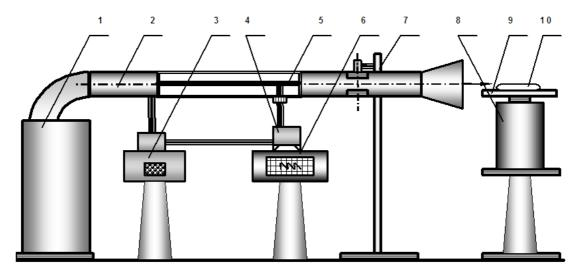
Figure 1: Experimental Laboratory Equipment for Drying of Low-Fat Milk in a Fixed Position on the Platform (Thin Layer): 1-Turbine; 2-Gas Pipeline; 3-High Voltage Impulse Generator; 4-Transformer for Increase The Voltage; 5- Electrode-Emitter; 6 -Electronic Oscilloscope; 7 - Tripod; 8-Electronic Weighing Device; 9 - Dielectric Platform; 10-Sample of Low-Fat Milk
