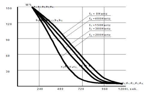
Figure 3: Drying Kinetics of Low-Fat Milk in a Thin Layer at Different Frequency Impulses: "A – B" – 1 Period of Drying, "B – C" – 2 Period of Drying, "C – D" – 3 Period of Drying
