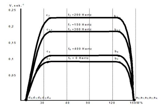
The General conclusion, that with the optimal speed  $V_0 = 0.220 \text{ sec}^{-1}$ , drying speed increased to 1.82 times.
